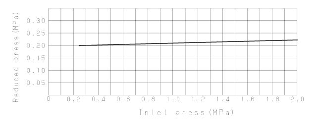
The above chart shows the change in the reduced pressure when the inlet pressure is changed in the range of 0.25  $\sim$ 2.0 MPa whereas the reduced pressure is set at 0.2 MPa at inlet pressure of 0.25 MPa.
