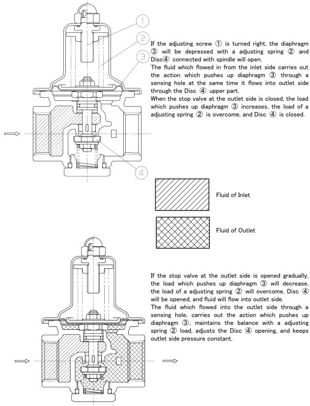
If the adjusting screw 1 is turned right, the diaphragm (3) will be depressed with a adjusting spring (2) and Disc④ connected with spindle will open.
