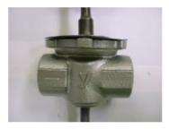
16) Place the adjusting screw on the adjusting spring.
