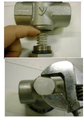
21) After adjusting the pressure, mount the hexagon cap nut on the thread of the adjusting screw.
