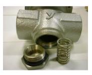
8) Applying, respectively but simultaneously, a socket wrench of nominal designation 10 to the U nut on the top of diaphragm and the hexagon nut on the valving element, remove the hexagon nut. Remove flat washer and then valving element P.
