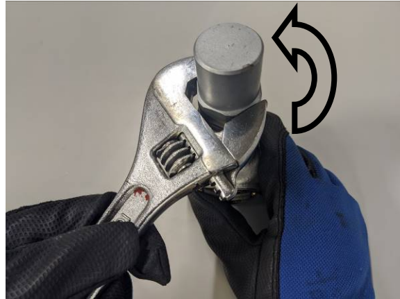
2. Remove the cap [11] with a wrench by turning it counterclockwise.
