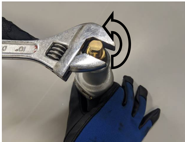
3. The lock nut [10] appears after you remove the cap [11]. Loosen the lock nut [10] by turning it counterclockwise with a wrench.
